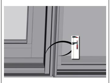
Place the units together making sure they are flush and level. Apply a hand clamp to keep the units together.
